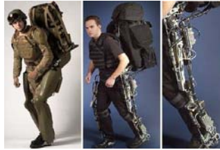
DARPA and the U.S. military are working on the Berkeley lower-extremity exoskeleton (Bleex). The exoskeleton system has two hydraulic leg braces that include 40 electronic sensors, a monitoring computer and an internal-combustion engine. The exoskeleton is attached to the legs of the soldier and allows for backpack loads upwards of 220 lb. to be carried with ease.
